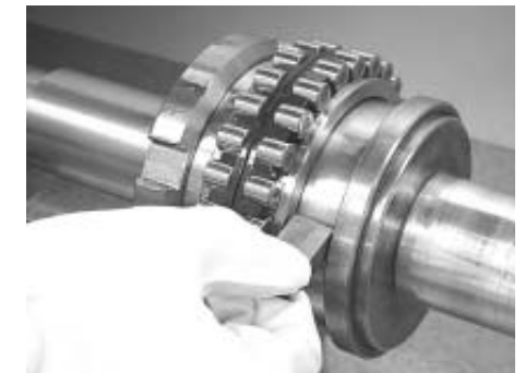
Fig. 1.15 Measurement of Spacer Width
