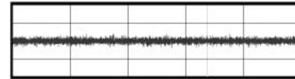
Sound waveform of a normal bearing
