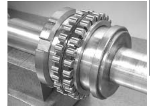
Fig. 1.13 Setting of GN Gauge
