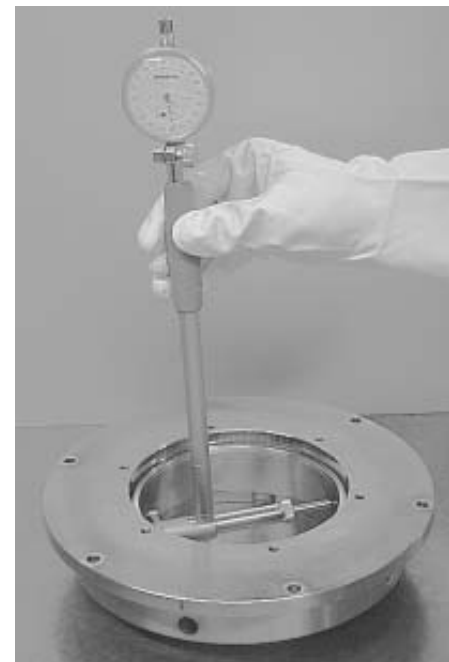
Fig. 1.10 Zero Setting of Cylinder Gauge
